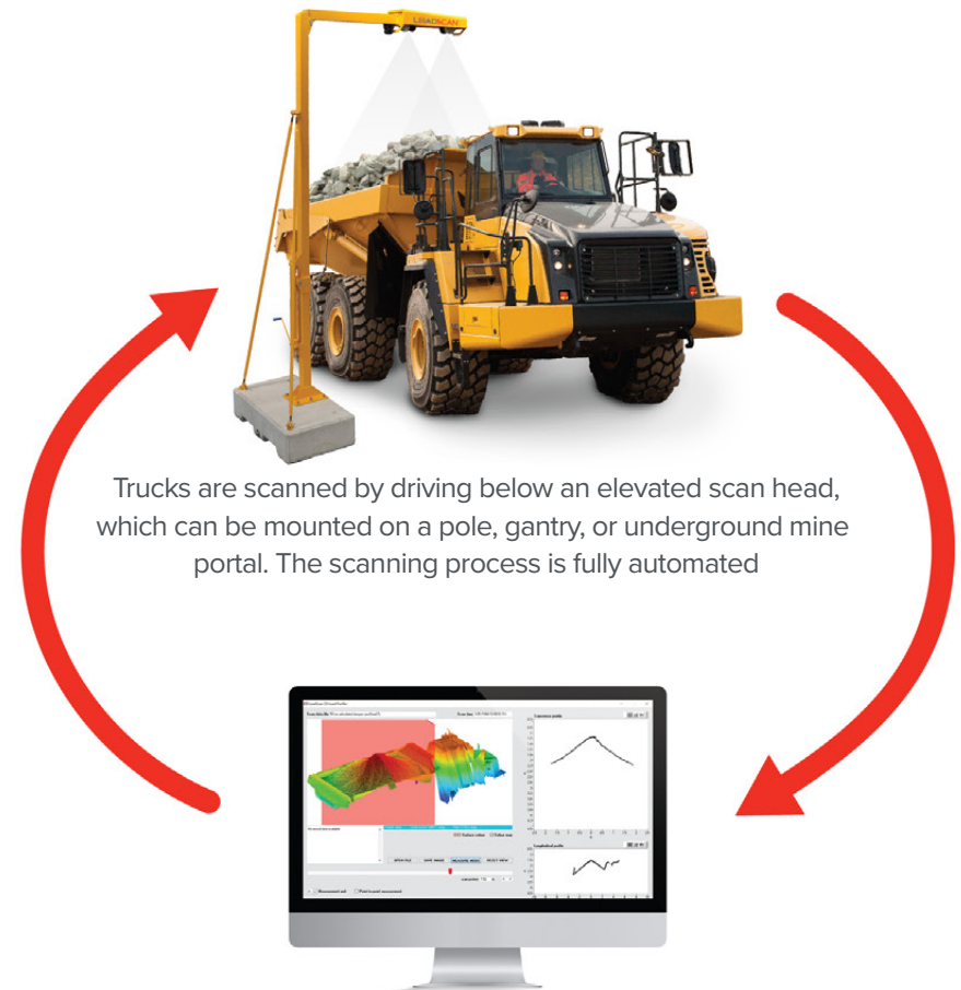
Proprietary Loadscan mining software reports volumetric measurement, including 3D load profiles of every load
